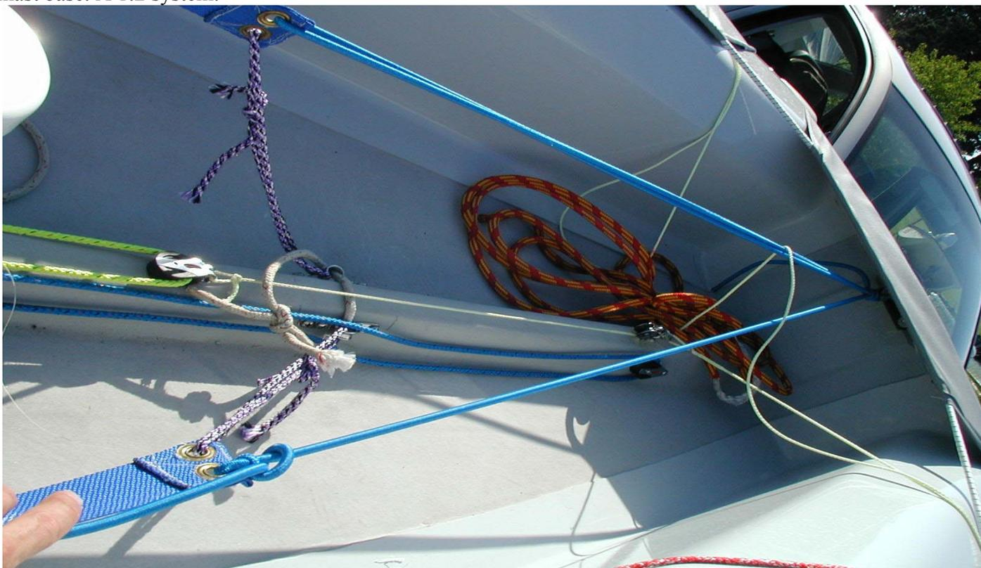
The photo below shows how the centerboard control is led as well as the vang and traveler controls. The red line exiting the trunk is the centerboard control the blue one on the other side on the trunk is the jib halyard tensioner. Also shown in this picture part of the jib sheeting system.
