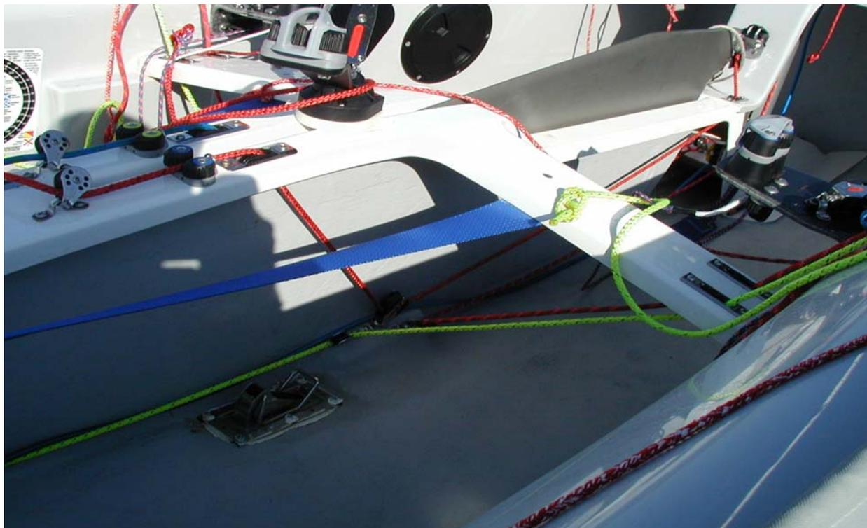
This picture shows the main halyard cleat mounted to the inside of the trunk upright. Also shown is the jib cloth tensioner.
